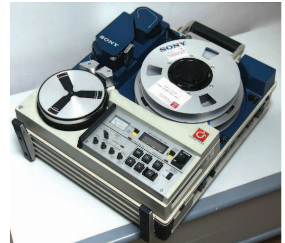
Sony's portable one-inch machine. Notice that the two tape reels are atop one another. These coaxial tape reels had the take up reel on top. The Ampex VPR-20 had the same configuration.
