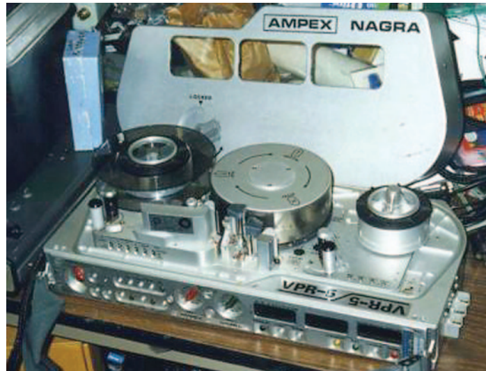
Portable one-inch VTR. This one was manufactured by Nagra, a well known audio recording company, which produced this machine in conjunction with Ampex. As the technical OEM, Ampex branded and sold it. Ampex offered an earlier version that was problematic, the VPR-20.
