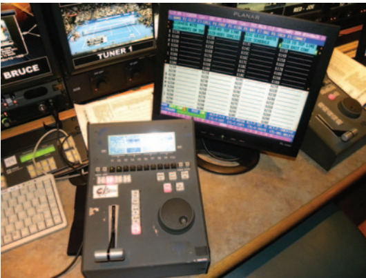
Generally, each IO channel in an EVS frame is controlled by an operator replay panel as shown here. Each panel has a RS-422 connection to a port on the EVS frame. An eight channel device would mean that up to eight of these control panels could be connected to a single box. To allow for flexibility, the control cables from each panel go through a patch panel or RS-422 router to allow any panel to connect to any control port on an EVS frame.
