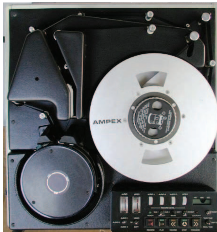
This was the Ampex original portable one-inch VTR, the VPR-20. It was introduced in 1979. It was aimed at the EFP market."
