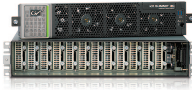
Here is the latest video server offered by Grass Valley, the K2, with the front cover off and sitting atop the unit. Like most things technical, it has gotten smaller and much more capable.
