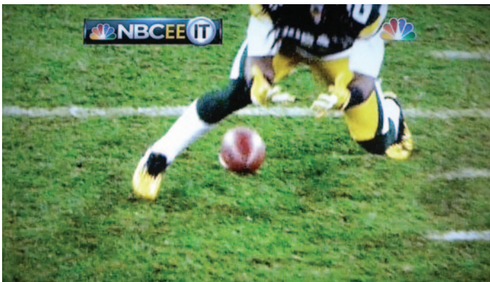
Screen shots showing 4K camera in a regular HD broadcast in a replay, and then the replay is stopped and zooms into the area of interest by eliminating most of the 4K pixels down to a point where only the desired number of HD pixels are used.
