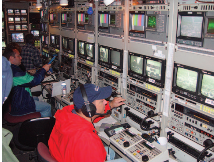
10 years ago, this tape or replay compartment, which consumed an entire trailer, was used for Monday Night Football. Here it is being used for the Indianapolis 500. Its usual complement was 16 VTRs and a few channels of EVS server storage. Today it is not unusual to have over three times the replay capability of this truck.
