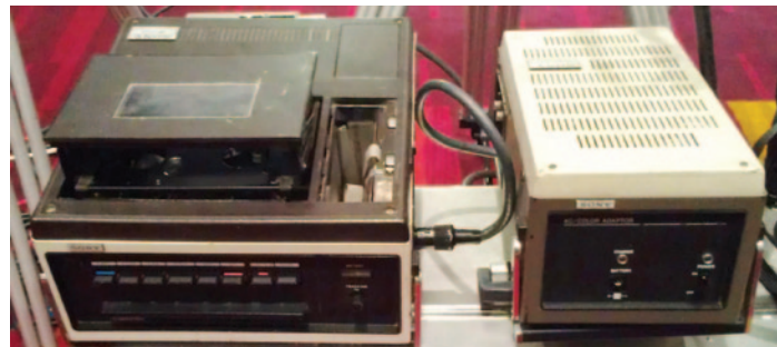
The VTR truly became portable with the advent of the \frac{3}{4} inch tape VTR, known generally by the Sony brand name Umatic. The machine shown here (on the left) was known as the VO-3800 (the box on the right is its optional power supply). This VTR was originally intended for industrial video use, but was adopted by innovative broadcasters for ENG use. It weighed less than 25 pounds, but with ENG cameras of the day, and battery belt, the photographer was lugging over 50 pounds of gear. Many a photographer that was used to shooting 16 mm film soon developed back problems.
