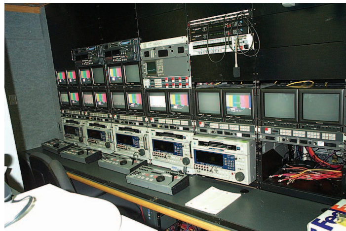
10 years ago, this was the replay compartment of a high end HD truck. The VTRs shown here, at their heart, were SD machines, but modified to be able to record and playback HD. The input and output of these machines had external MPEG encoders/decoders. The data laid down on tape was simply MPEG compressed audio/video. Today, most HD VTRs do the same, except the compression and decompression are built into the machine.
