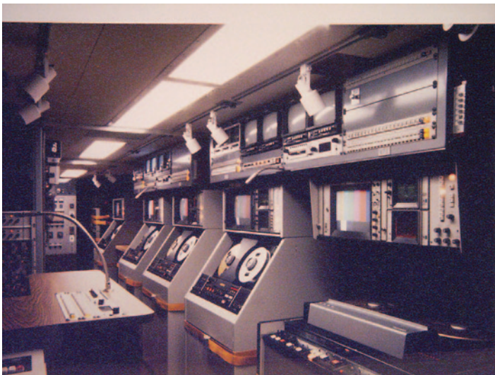
Here is a CBS owned truck in the early 1980s. This trailer only housed VTRs and an Ampex disk-based slo-mo system. As can be seen here, the transition from 2 inch VTRs (machine in the foreground) to one-inch VTRs is occurring.
