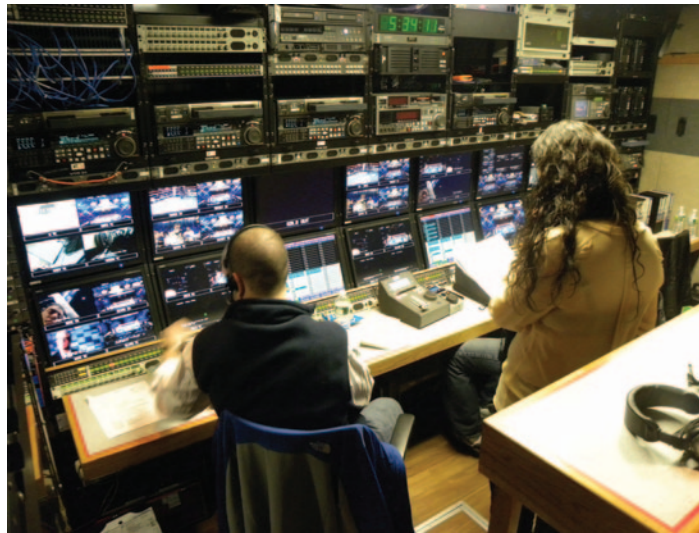
Even today the average replay compartment on a truck carries a combination of video servers and VTRs, as can be seen above the monitors.
