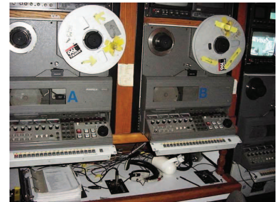
The machines here were once high end mainline VTRs used for recording and replay. These machines used one inch wide tape. They produced higher quality video than two-inch VTRs. They also played at speeds up to two times real time, down to stop motion, even slow reverse. One inch machines were the workhorses through the 1980s and into the 1990s.
