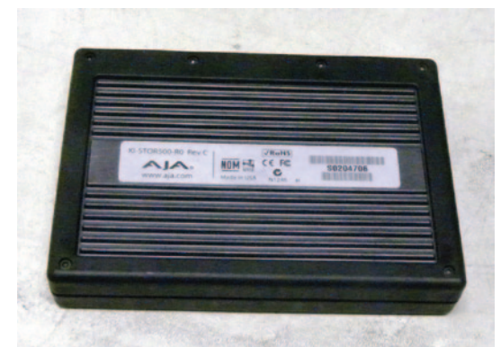
Here is another small, hand-held, storage module from AJA. It has 500GB of storage and spins at 7200 RPM. It works in conjunction with AJA's KiPro record/playback unit, which retails for under $5000.
